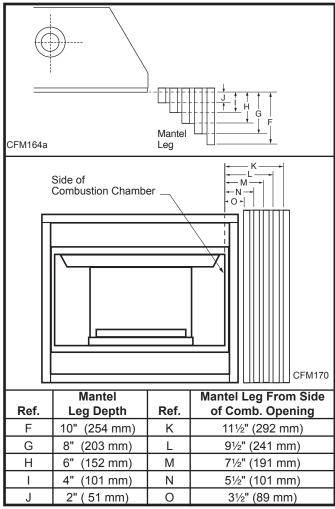
Fig. 3b Combustible mantel leg minimum installation.
